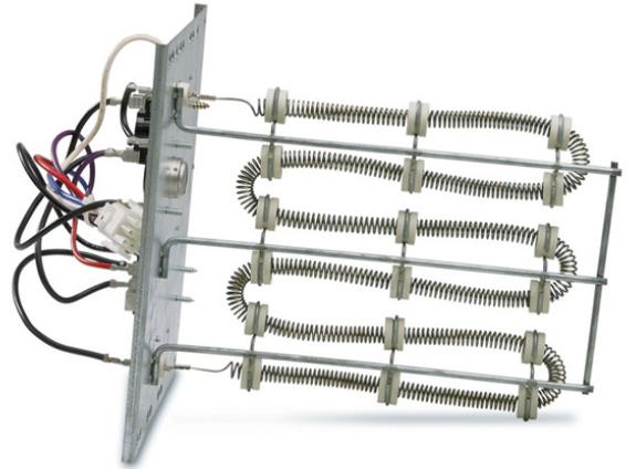
Open coil heater elements are supported by a ceramic insulators, used to isolate the resistive heating elements. They provide an economical means of heating inert or non-corrosive gases when a protective sheath is not required.
